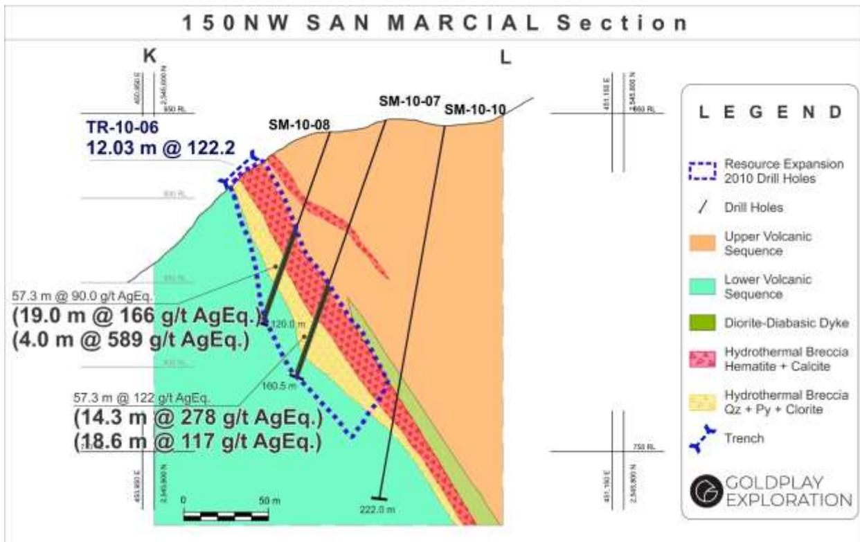
Figure 3: San Marcial Cross Section I-J
