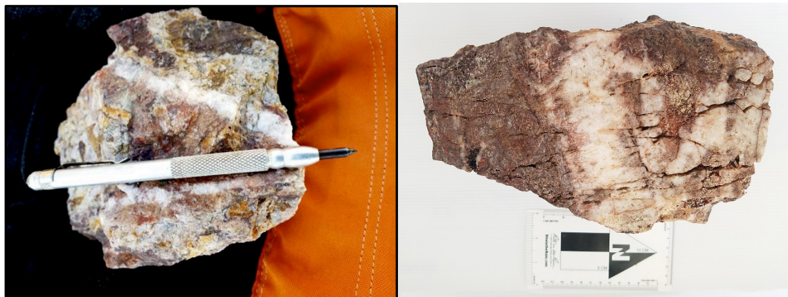
Figure 5 Nava Zone – Epithermal Stockwork Quartz Veinlets with Boxworks of Hematite (ex-Pyrite)
