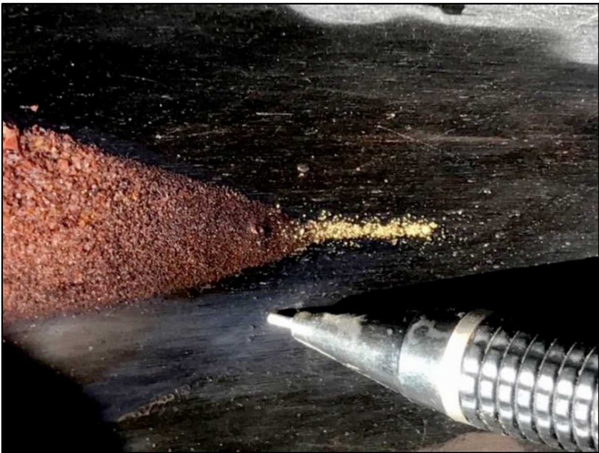
Figure 1 Visible Gold from Panning of Epithermal Quartz Vein Channel Sample – Nava Zone (1)
