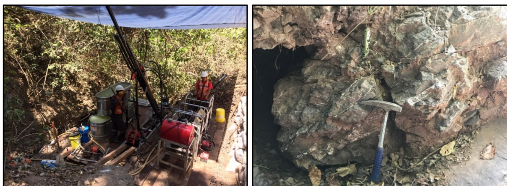
Figure 3: Chachalaca Target – (a) NW150 Diamond Rig and (b) a Swarm of Quartz Veinlets
