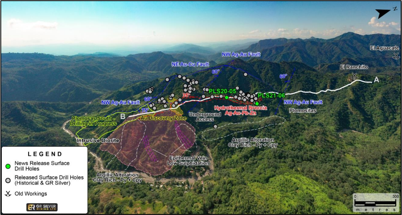
Figure 1: Drone Image - Plomosas Mine Area, Surface Drill Collars and the New Drilling Area known as Plomosas South
