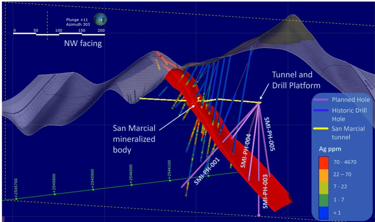
Targeting of the drill program was aided by 3D chargeability, resistivity, and magnetic inversion data products received by the Company over the Resource Area. Several zones of elevated chargeability correspond with volcanoclastic-sedimentary units that are found in the immediate footwall of the San Marcial Fault, overlapping with areas of disseminated pyrite, and coincident with previously reported gold intercepts (see [News Release dated November 12, 2020](#)).
