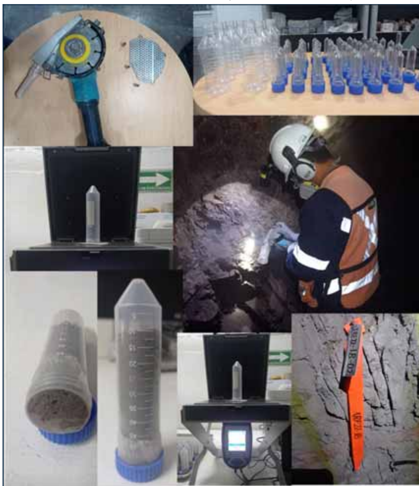
Figure 9-12: Plomosas Mine—Channel Sampling with Powder Recovery for pXRF Analysis
