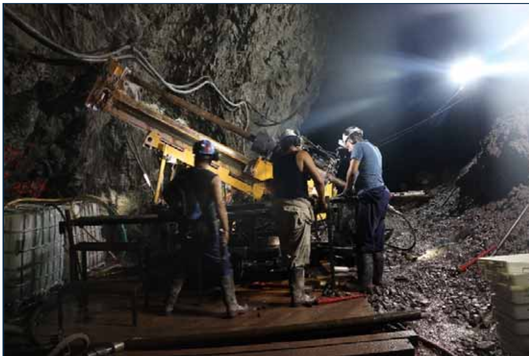
Figure 10-13: Boart Longyear LM 75 Owned and Operated by Intercore—at Plomosas Underground Level 833
