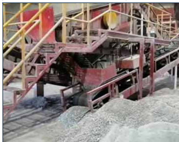
Figure 13-5: Crushing of Bulk Sample and Piling of Crushed Material at the Processing Plant
