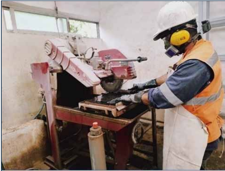
Figure 11-3: Cutting Core with a Diamond Saw at the Plomosas Core Shed
