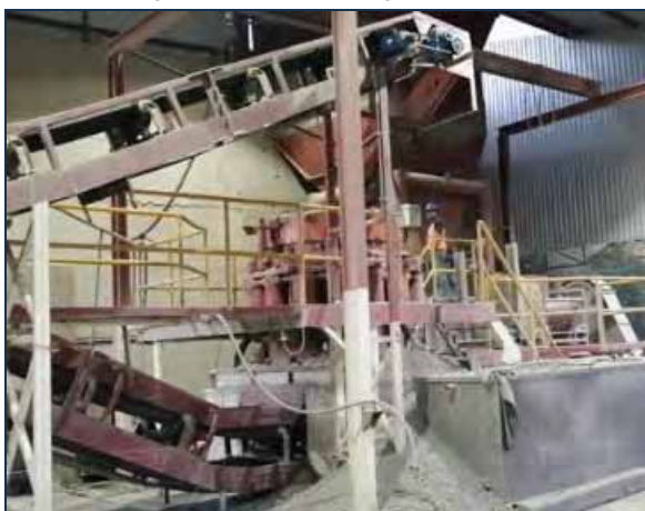
Figure 13-5: Crushing of Bulk Sample and Piling of Crushed Material at the Processing Plant
