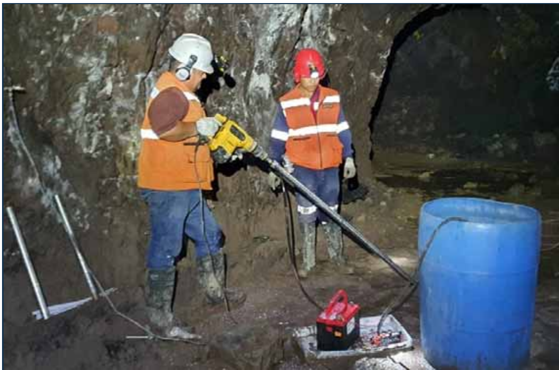
Figure 10-16: Portable Drill Rigs Operated by GR Silver—at Plomosas Mine Area Underground
