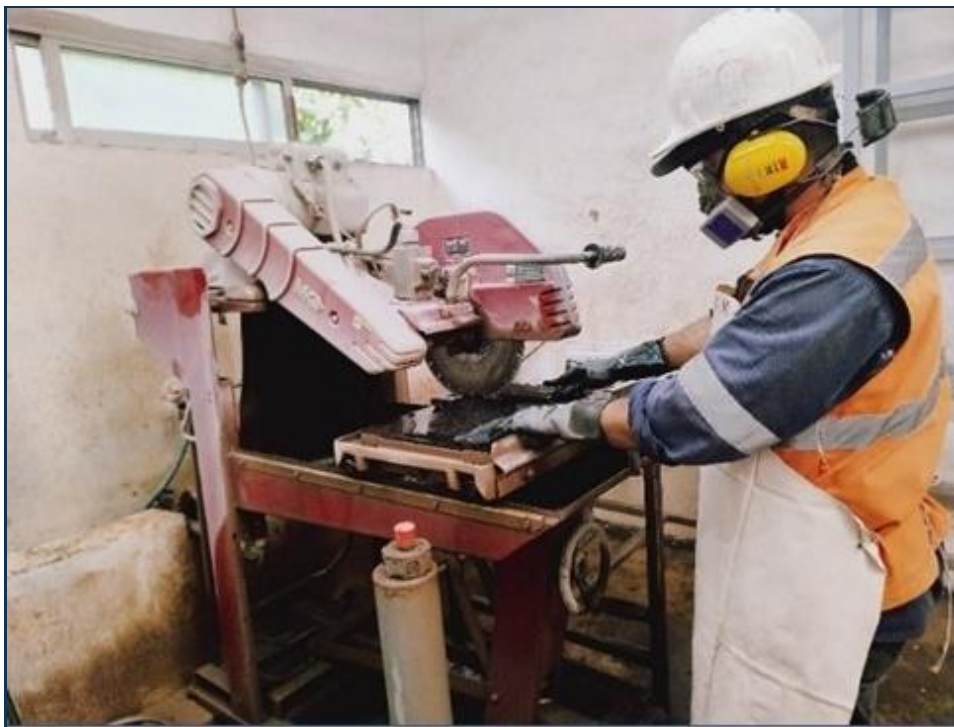
Figure 11-3: Cutting Core with a Diamond Saw at the Plomosas Core Shed
