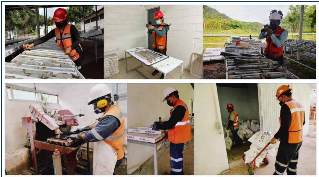
Figure 10-21: Core Logging, RQD, Core Cleaning, Photography, and Core Cutting at the GR Silver Core Shed Facilities at Plomosas
