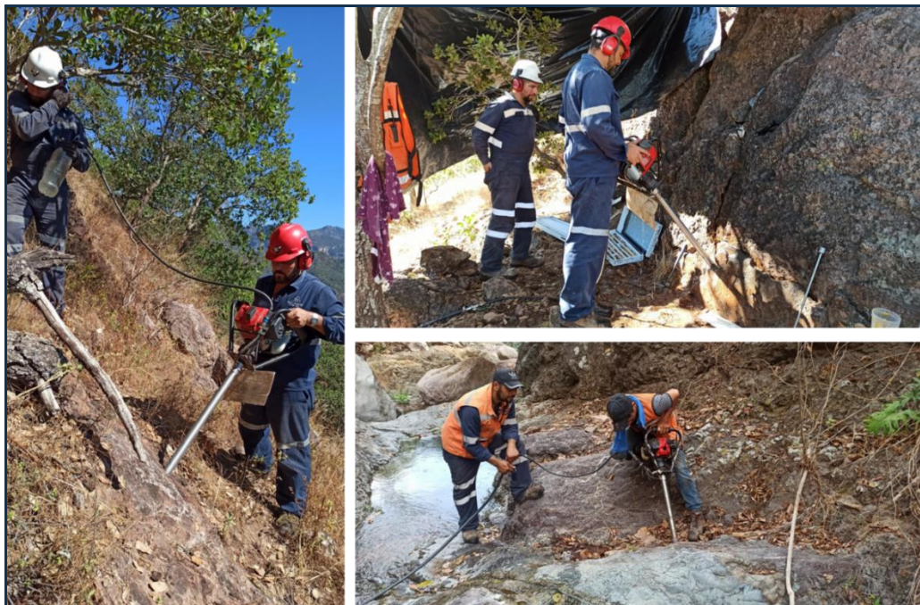
Figure 10-28: Adapted Portable Drill Rig to Difficult Access Areas at Surface
