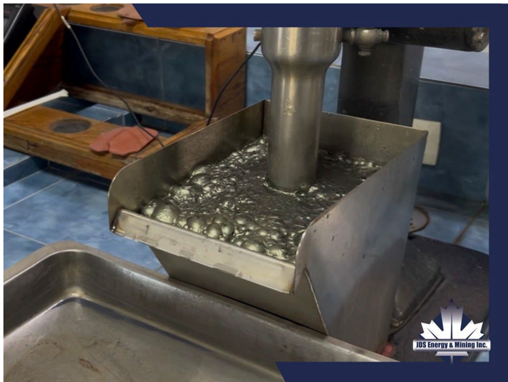
Figure 1 – Flotation Test Work – Cleaner Pb Concentrate Composite Sample
