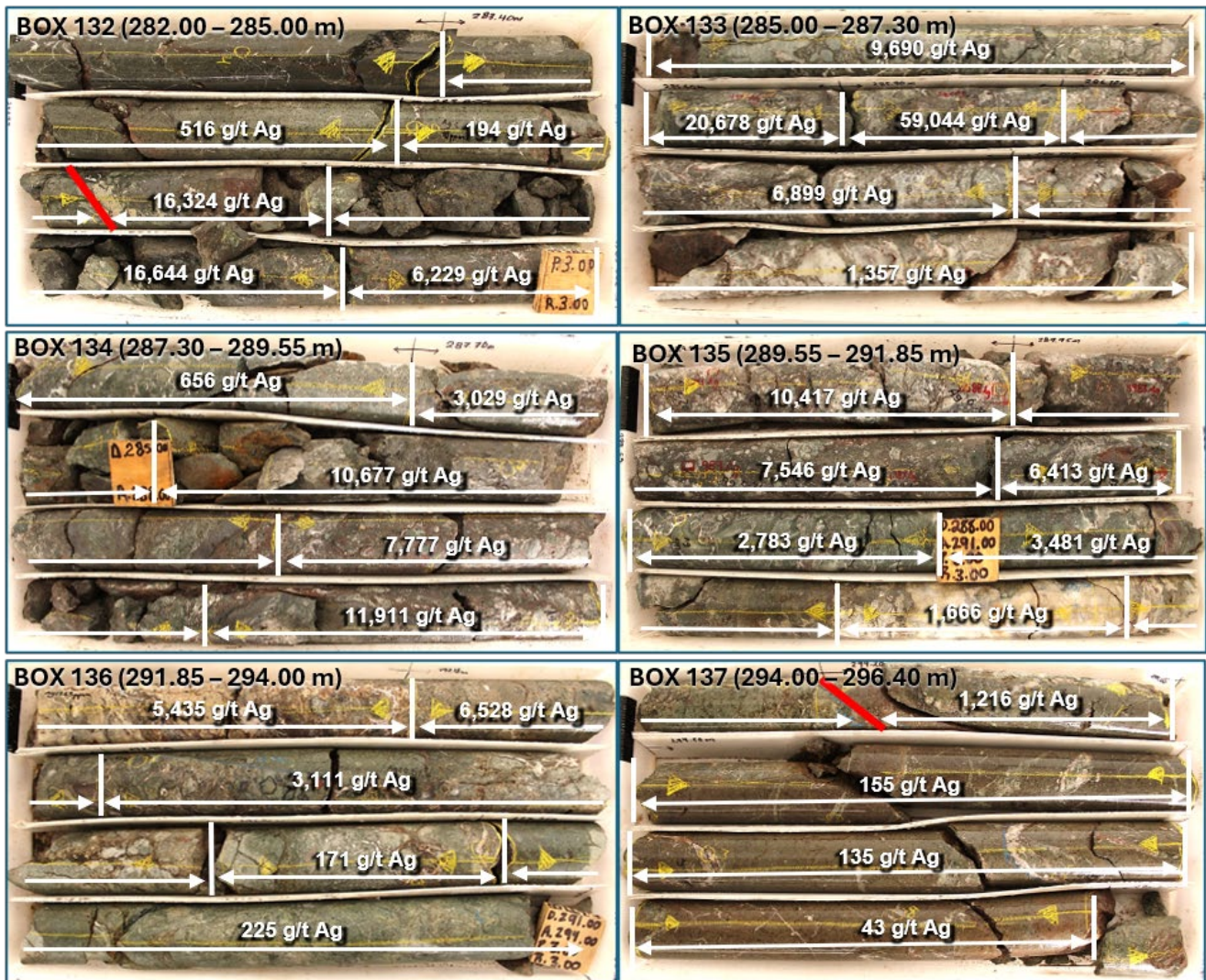
Figure 3 Drill Core Photo Illustration - SMS26-04 High Grades in Main Breccia Zone (Main breccia zone defined by red lines)
